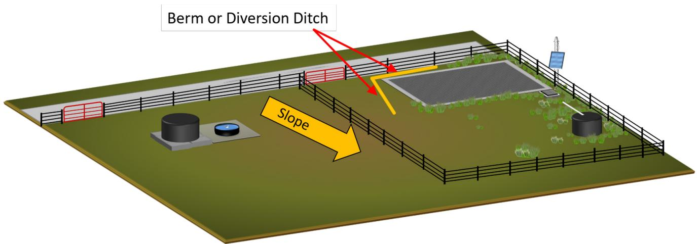
**Figure 4.** A rain trap with an upland diversion created to redirect flows that may contain pollutants. (Illustration by Donnie Stamper)
