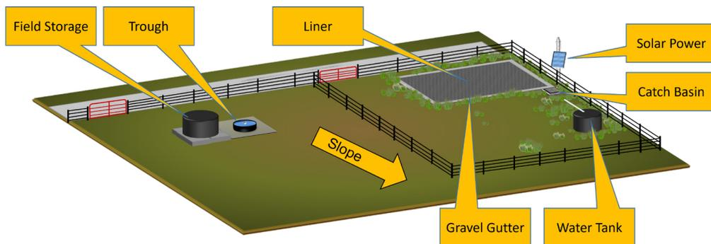
Figure 3. A solar-powered rain trap. (Illustration by Donnie Stamper)
