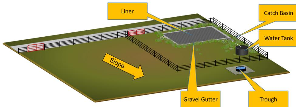
Figure 2. A gravity-fed rain trap. A fence excludes livestock from the trap. (Illustration by Donnie Stamper)
